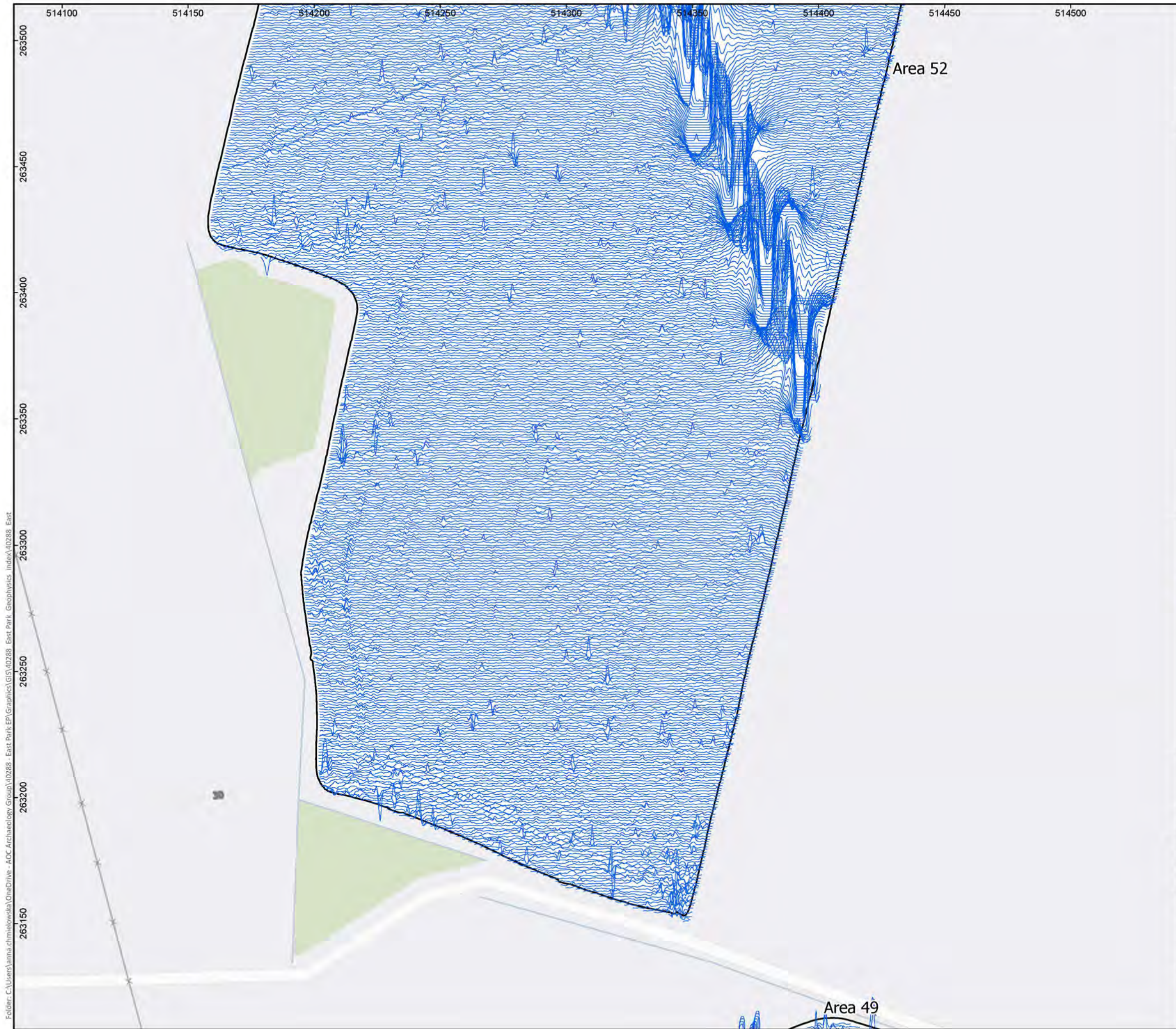
Figure 7.60 Minimally Processed Gradiometer Data – XY Trace
